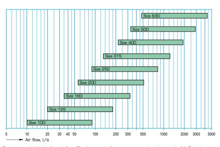
Recommended limits for air flow. The lowest air flows correspond to air speed of 1,5 m/s, which is the recommended minimum air flow to fulfil the  $\pm 10\%$  measuring accuracy.
